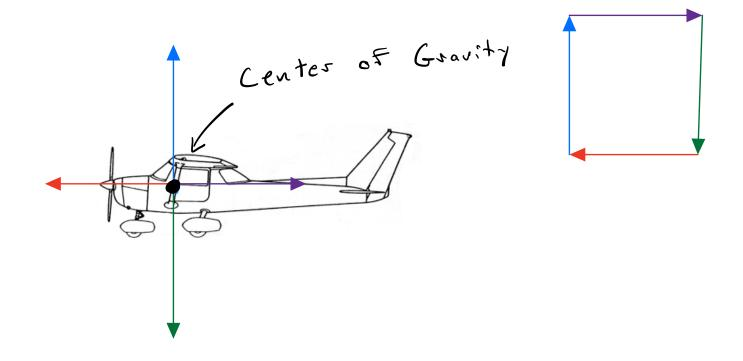
Fnet = 0 for unaccelerated flight
