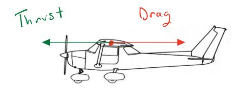
Thrust = drag in unaccelerated flight
