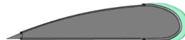
**FIGURE 3-2. CLEAR ICE BUILDUP WITH HORNS**
