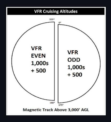
Above 3000' AGL, VFR traffic in level cruising flight shall fly:
